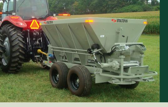
All Stoltzfus Wet Lime Spreaders can be configured with hydraulic drives. Your choice of manual controls or Variable Rate Ready (compatible with most controllers).
