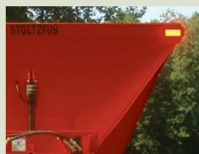
Steep, 53° hopper side slopes eliminates damp lime bridging on the RC-8010 and 45° side slopes on the RC-8012 allow higher capacity for fertilizer and other more flowable materials
