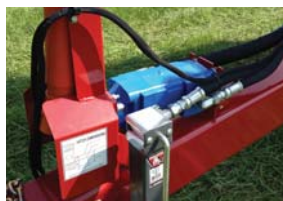
Self-contained PTO hydraulics reduces the strain on your tractor's hydraulic system
