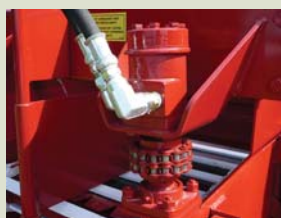
Spinner motors are mounted out of the flow of corrosive materials for increased life
