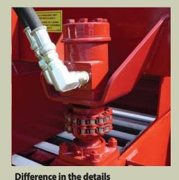
Attention to details like placing the spinner motor above the material flow not only keeps it out of harmful chemicals but also isolates the motor from the shock of material pounding on the spinner disk.
