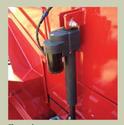
**Electronic gate actuator** Open and close the metering gate from the comfort of the tractor seat.
