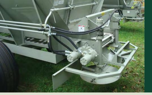
All Stoltzfus Bulk Material Spreaders can be configured with hydraulic drives. Your choice of manual controls or Variable Rate Ready (compatible with your Raven controller).
