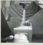
**Optional shredder** Heavy duty blades chop up any clumps and gives a smoother flow of material onto the spinners.
