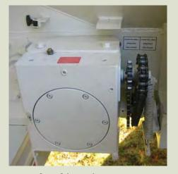
Heavy duty drive train Proven PTO drive system and dual speed drives eliminates slipping.
