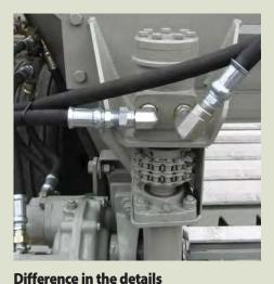
For example, placing the spinner motor above the material flow reduces exposure to corrosive materials. Furthermore, it eliminates vibration and isolates the motor from the shock of material pounding on the spinner disk.
