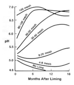
Figure 2. Reactivity of lime as affected by particle size.
